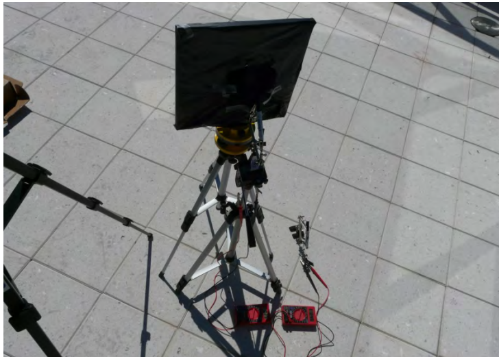
Figure 6. The measurement of the reference sample on the 35 th floor. The pyranometers read 245 (sensor in direct sun) and 25 (sensor sees the sun via the reference sample).
