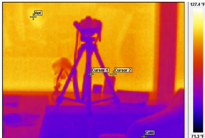
Figure 11. The suite # [REDACTED] at 10:34am on [REDACTED]. The glass measurements and the tripod with the camera recording the measurements photographed in the long IR range. Note the approx. 127 °F radiation.
