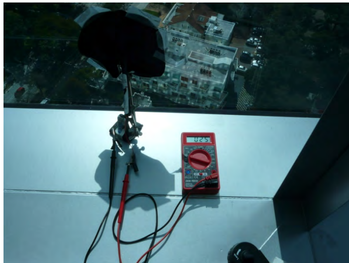
Figure 7. The pyranometer measuring the glass pane #2 in suite # █.
