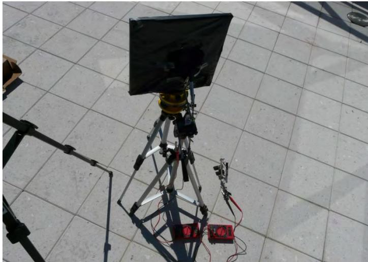
Figure 6. The measurement of the reference sample on the 35<sup>th</sup> floor. The pyranometers read 245 (sensor in direct sun) and 25 (sensor sees the sun via the reference sample).
